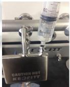
Replace cap, by Depressing spring side of Clip, and pressing Opposite side to lock into Place, one the cap has Been fitted to the Coupling.
