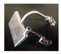
The Clip-On Steamer is designed to use an external heat source such as a torch to heat the small rectangular vessel to produce steam.
