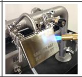
Avoid contact with the Keofitt quick-couplings As they contain silicone orings And will Deteriorate with direct Flame to their contact Parts.
