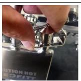
Apply torch flame to Upper third of vessel, and Move side to side until Water vapor / steam Appear, work your way Down from the top, as the Water level decreases. Steam for 1 minute or to Standard operating Procedure.
