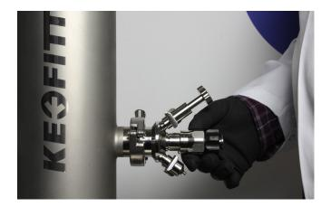
7. Release the handle on the Emergency Tool by turning it 90 degrees and slide into the groove of the holder.
