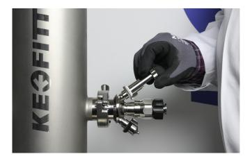
14. Valve head is now assembled to the valve body. Use the Tommy bar to tighten.
