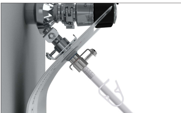
PICTURE 7. Quick Coupling KSB Outlet 3/8” Hose barb (#150082) mounted on the KEOFITT Sampling Bag™ outlet. KEOFITT Sampling Bag™ is mounted on Sesame sampling valve. When cleaning, disinfecting, or sterilizing the pinch clamp must be open to allow for passage of the media (left). Immediately after cleaning, disinfecting, or sterilizing, the pinch clamp must be closed to avoid contamination of the interior (right).
