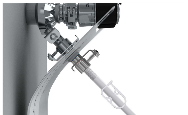
PICTURE 7. Quick Coupling KSB Outlet 3/8” Hose barb (#150082) mounted on the KEOFITT Sampling Bag™ outlet. KEOFITT Sampling Bag™ is mounted on Sesame sampling valve. When cleaning, disinfecting, or sterilizing the pinch clamp must be open to allow for passage of the media (left). Immediately after cleaning, disinfecting, or sterilizing, the pinch clamp must be closed to avoid contamination of the interior (right).
