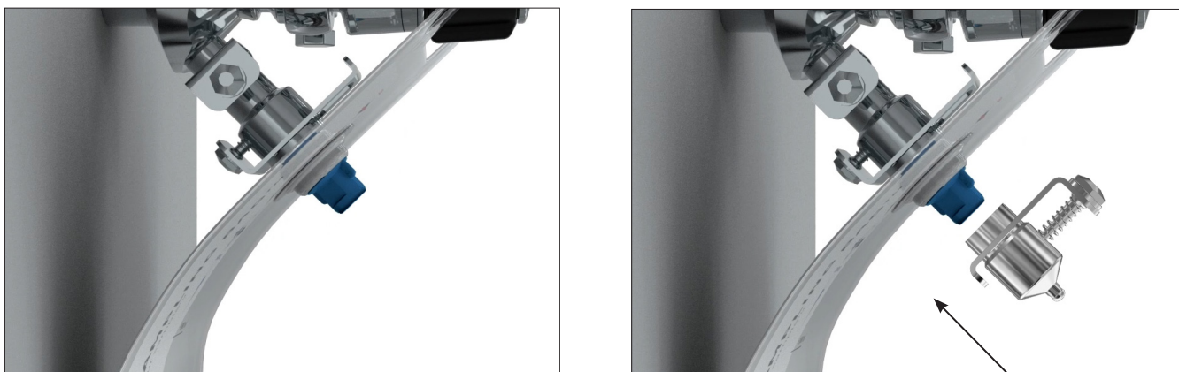
PICTURE 8. Left: Protecting aluminium foil removed from the outlet for a free flow path of the cleaning, disinfection, or steam media. Right: Immediately after cleaning, disinfecting, or sterilization, mount the Quick Coupling KSB Outlet stainless steel plug. It is recommended to disinfect the stainless steel plug just before mounting.
