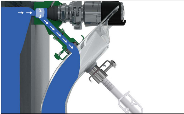
PICTURE 12. KEOFITT Sampling Bag™ in sampling position. The product flows through the valve into the open KEOFITT Sampling Bag™. Quick Coupling KSB Outlet 3/8" Hose barb (#150082) is mounted on the outlet of the KEOFITT Sampling Bag™.
