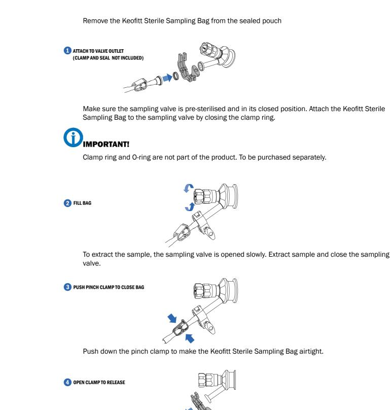
Disconnect clamp ring and remove the Keofitt Sterile Sampling Bag.
